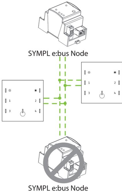
Do not leave any wires open! Open wires will cause signal reflections and therefore disrupt communication.
