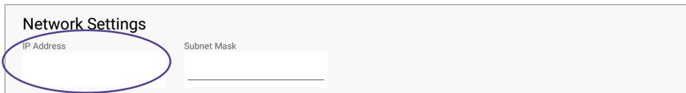
Unique IP address; must be coordinated with the rest of the Ethernet network settings.
