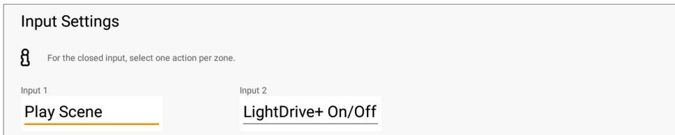
For both digital inputs individually, you can select the reaction of the LIGHTDRIVE+ on closing the input.
