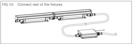
5. Use interconnection cable if fixtures are not adjacent to each other. Plug the end cap to the final fixture of the chain to complete the connection. Connect the starter cable to AC power.
