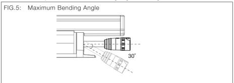
• 4 feet version cables have a minimum bending radius of 30mm.
