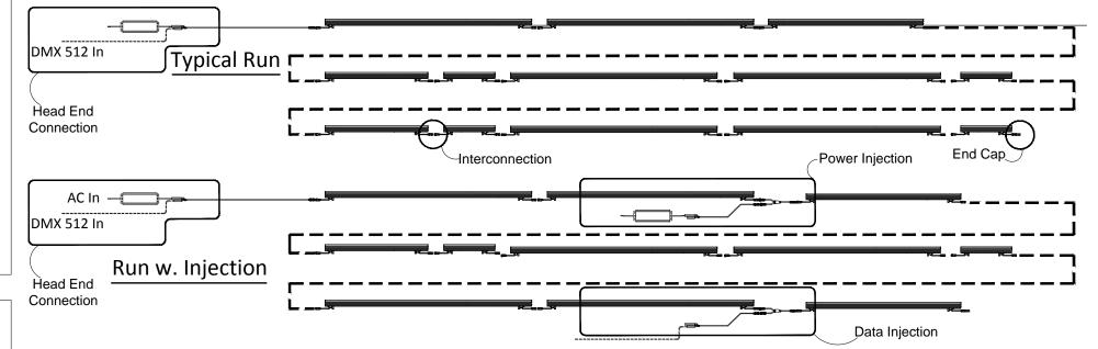
Maximum length of interconnected LED tubes on a 100w power supply is 20'.
