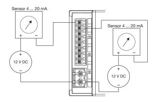
When connecting multiple 2-wire sensors, each must have its own power supply.
