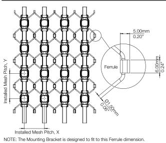
High Density Dot Media Solution - STAINLESS STEEL MESH GRID
