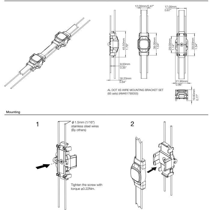
Low Density / Single String Installation Solution - WIRE MOUNTING
