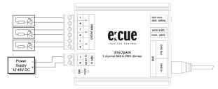
The advantage of the above shown type of connection is the reverse supply protection of all LED fixtures and the dimmer itself. Alternatively it is also possible to connect LED fixtures as shown in the figure below.
