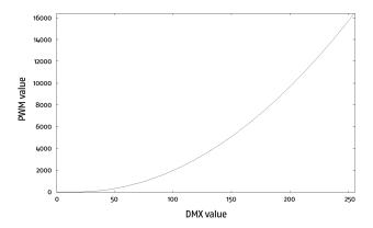
The dimming of the LEDs is accomplished by a pulse width modulation with a basic frequency of f=488 Hz. Due to the 14 bit PWM resolution, the "On-time" can be adjusted in 125 ns steps. To achieve a more "linear" impression of the LED's brightness, a translation from the 8 bit DMX value to the 14 bit PWM resolution in form of a dimming curve is implemented.
