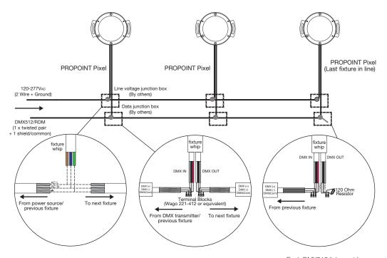
Each DMX512 link must be properly terminated to prevent signal reflections.
