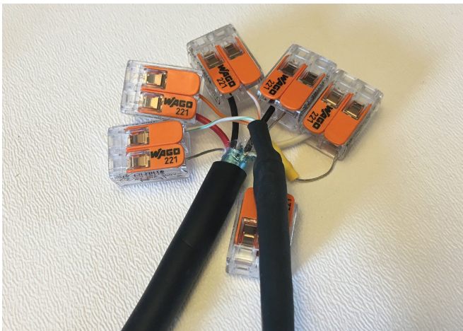
Figure 23 – DMX Termination Detail
