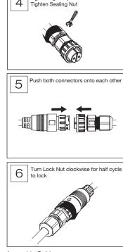
Tightening Torque:  $0.7-0.9 \mathrm{Nm}$
