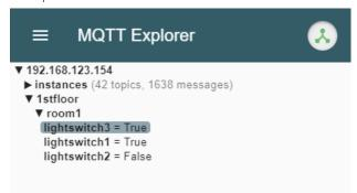
In the "MQTT Explorer", enter the following settings to connect to the MQTT broker in SYMPHOLIGHT:
